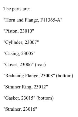
The front nuts are 42236, the rear 42235 and the bottom flange 44468. No numbers are given for the front and rear gaskets.
